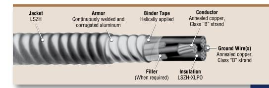
LSZH XLPO Insulation Aluminum Armor LSZH Jacket **UL** Listed 90°C\*, 600 Volt **NEC Type MC** NFPA 130 & 502
